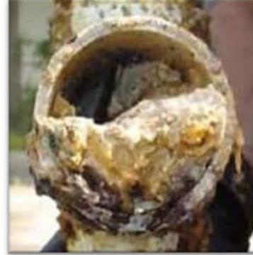
Clogged Sewer Line Caused by FOG
